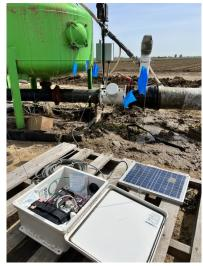
**Figure 2**. A flow meter was connected to communication devices in a processing tomato field in Crows Landing, CA (photo taken on April 17, 2023). Utilizing the flow meter, datalogger, and cellular modem, we can access to field irrigation data remotely through CropManage while offering irrigation recommendations to growers.
